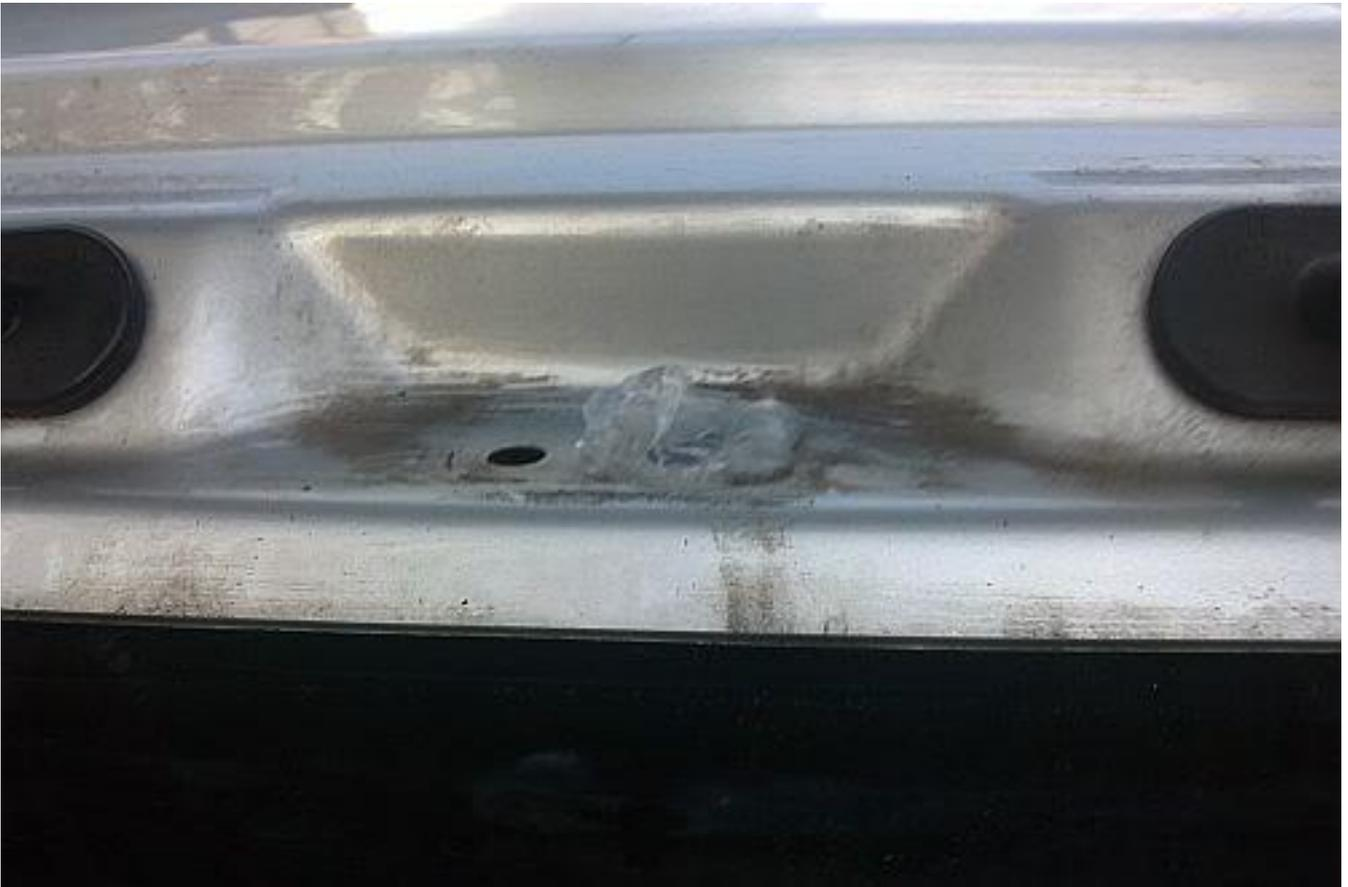
**Bolt hole on hatch with clear silicone sealant applied**
