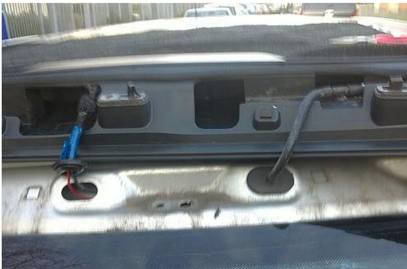
Underside of old spoiler showing bolt holes, washer pipe (right) and wiring (left) the blue tape is where I attached the wire for my rear badge brake LED light.
