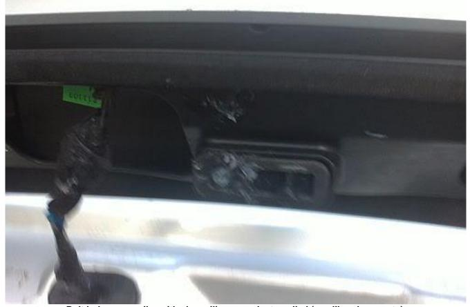
Bolt holes on spoiler with clear silicone sealant applied (use liberal amounts)
