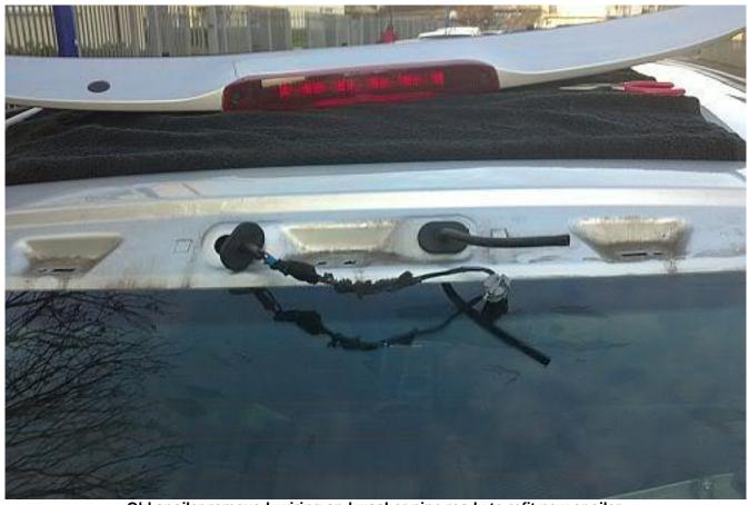
Old spoiler removed, wiring and washer pipe ready to refit new spoiler
