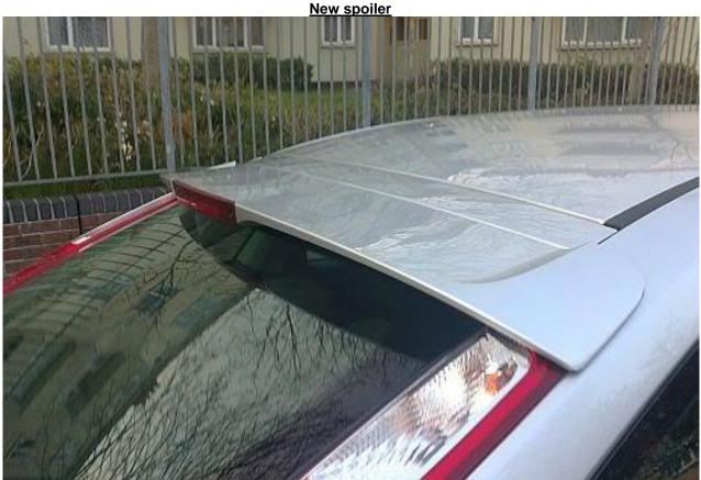
If you were looking to fit a ST spoiler, then the process is exactly the same except the wire connector is different so will need splicing to a new one (the brake light is a different shape).
