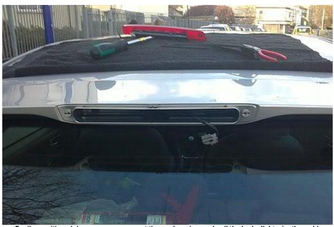
Spoiler positioned, (ensure you reconnect the washer pipe, and pull the brake light wire through)
